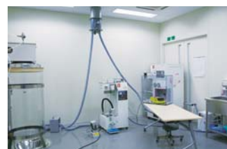
Spray Dry Laboratory We take all accepted various samples, like food, organic chemistry, or inorganic chemistry and will measure the particle size and recover rate after powderization.
