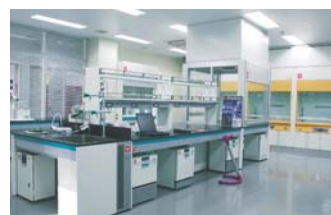
Fume Hood and Air Conditioner System Evaluation Laboratory At this laboratory, we reproduce air-control systems in a Fume Hood as well as the entire laboratory in order to confirm certain enclosures for the appropriate air pressure and exhaust. Additionally, it functions as the showroom for the whole laboratory.
