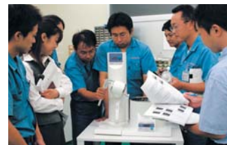
Trial Room (Exam and evaluate every manufactured instrument) Each new product goes through various evaluations and environmental testing using the latest technology. In addition, the latest in air flow management is used in examinations to test wind velocity, air current, and leakage based on the standards put forth in the American Society of Heating, Refrigerating and Air-Conditioning Engineers (ASHRAE).
